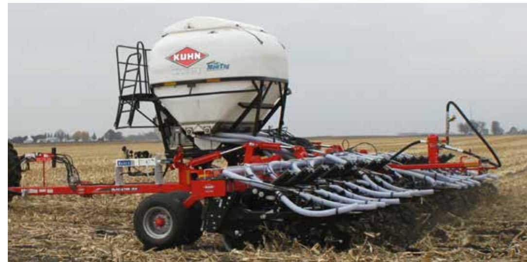
Gladiator 1210 pull-type models are all available with either 6-ton or 9-ton dry fertilizer tanks or a 1,000 gallon liquid tank mounted on the chassis.
